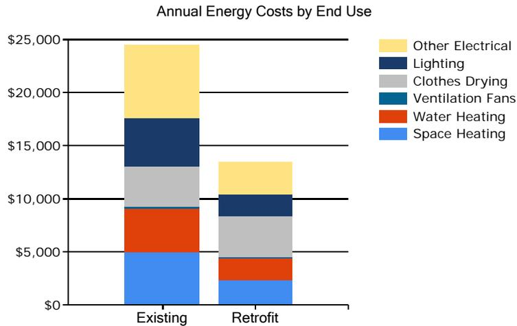
Figure 3.2 below shows how the annual energy cost of the building splits between the different fuels used by the building. The “Existing” bar shows the breakdown for the building as it is now; the “Retrofit” bar shows the predicted costs if all of the energy efficiency measures in this report are implemented.
