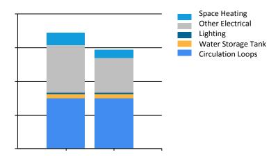
Figure 3.2 below shows how the annual energy cost of the building splits between the different fuels used by the building. The "Existing" bar shows the breakdown for the building as it is now; the "Retrofit" bar shows the predicted costs if all of the energy efficiency measures in this report are implemented.
