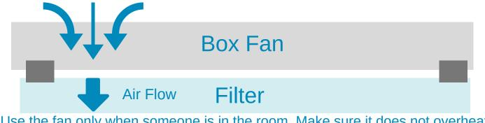
3. Use the fan only when someone is in the room. Make sure it does not overheat.4. Replace filter when dirty.
