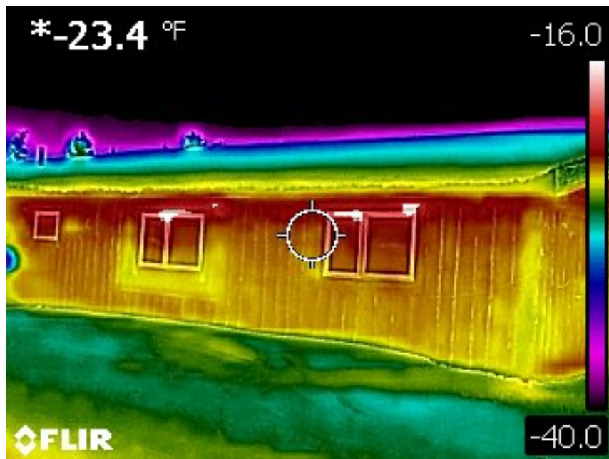
FLIR thermal imaging of the side of the building. The color gradient on the right depicts the temperature range of the photo (-40° F to -9.9° F). The window sashes are not well-insulated (white areas above the window panes).
