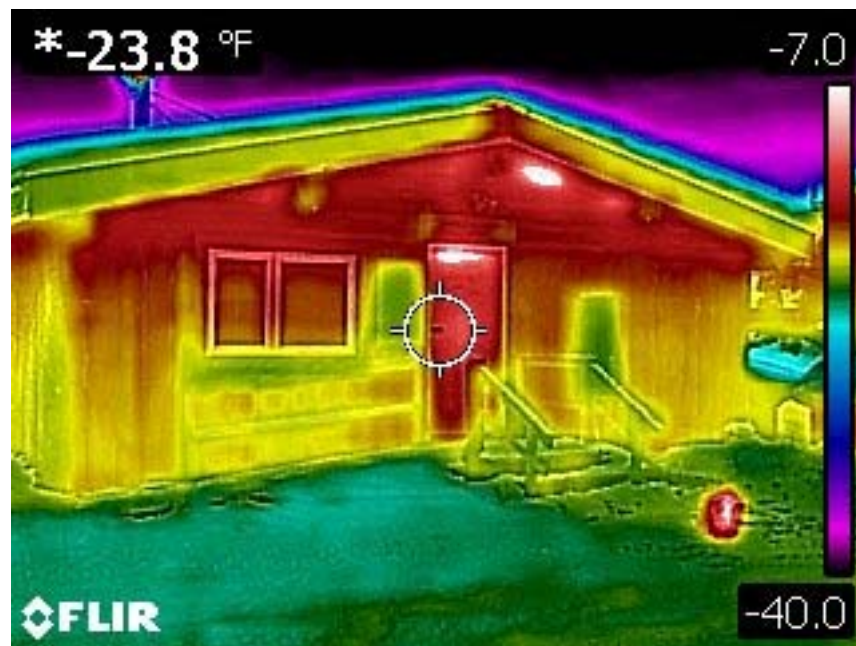
FLIR thermal imaging of the building main entrance. The color gradient on the right depicts the temperature range of the photo (-40° F to -7° F). Colors in the higher end of the gradient indicate where heat is being lost. The red spot on the ground in front of the building is a cat.
