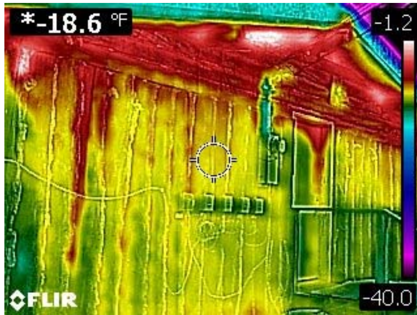
Close up thermal image of the building's rear exit. The color gradient on the right depicts the temperature range of the photo (-40° F to -1.2° F). Note the areas of heat emission (white) at the roof and the left corner of the wall.
