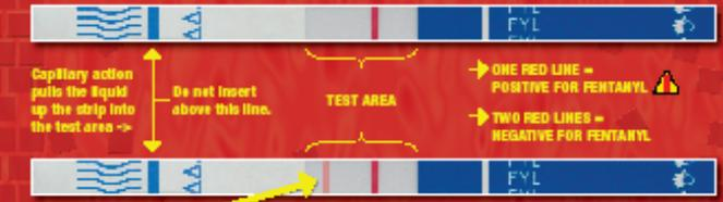
Capillary action pulls the liquid up the strip into the test area →
