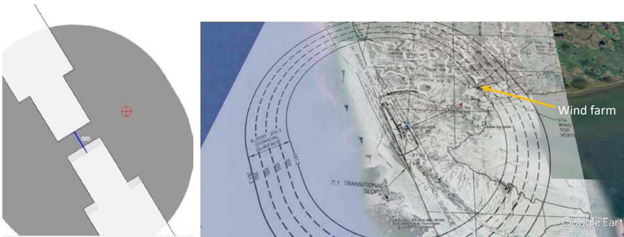
Figure 10: FAA obstruction evaluation result and Hooper Bay Airport Layout Plan overlay on Google Earth imagery
